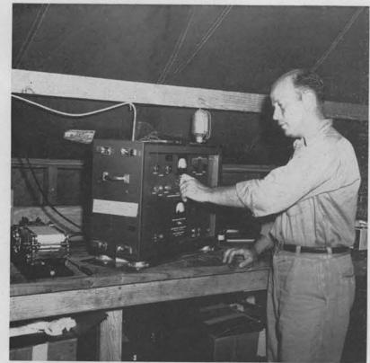
EQUIPMENT TEST-Gus Gustafson, formerly of 5232, checks the microbarograph amplifier and recorder at the station on Ujelung.
